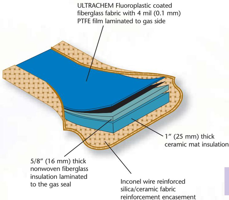
**FLEXON-1500** A composite belt designed to provide continuous service at elevated continuous temperatures to 1500°F (816°C).
