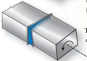
**Axial Compression/Extension** - The dimensional shortening (compression) or lengthening (extension) of the expansion joint face-to-face dimension parallel to its longitudinal axis.
