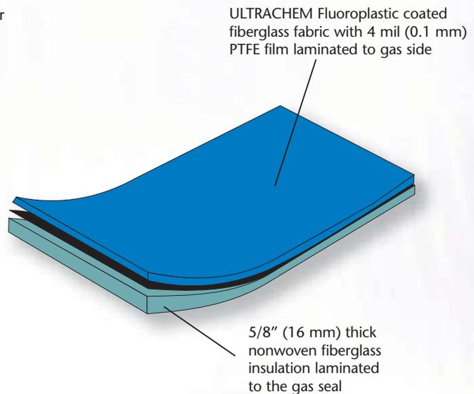
**FLEXON-1200** A composite belt designed to provide continuous service at 1200°F (649°C), by the addition of a 1/2" (13 mm) of ceramic mat insulation to the FLEXON 1000. Inconel® wire inserted silica cloth is used as the encasement to replace fiberglass in applications above 1000°F (538°C).
