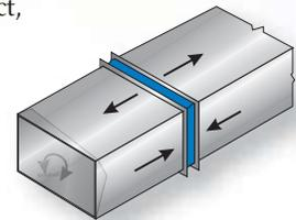
**Torsional Deflection** - The amount of twisting movement (in degrees) occurring in the perpendicular planes to the longitudinal axis of the duct system.
