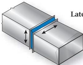
**Lateral Movement** - The amount of duct movement occurring in either or both of the two perpendicular planes to the longitudinal axis of the duct, which moves the expansion joint flanges out of alignment.
