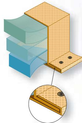
Typical cavity pillow construction consisting of layers of insulation encased in a protective high temp sleeve.
