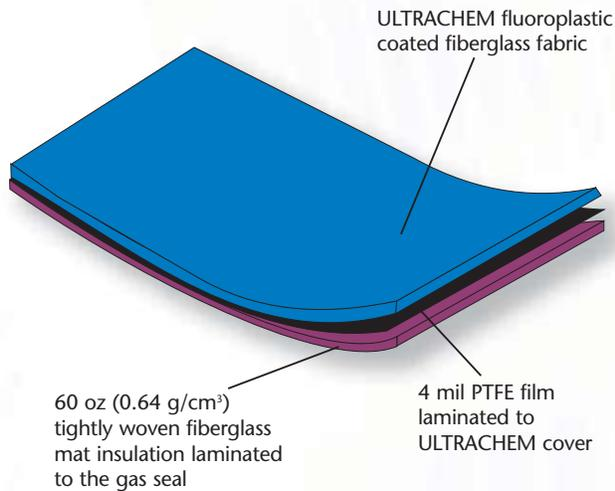
**FLEXON-700** A composite belt designed to provide continuous reliable service at 700°F (371°C). A tightly woven fiberglass insulation is thermally bonded to the FLEXON material. This composite design provides insulating properties at elevated temperatures and prevents separation of the insulation.
