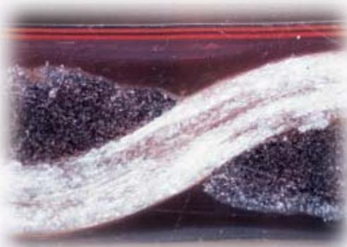
Perfluoroplastic, due to its crystalline nature, is inherently stiff which reduces the long term flex endurance and life of PTFE fabric expansion joints. To overcome this shortcoming, fluoroelastomer (Viton®/Fluorel®) is blended into a patented alloy which bathes the coated fiberglass matrix significantly increasing the flexibility, tear resistance, tensile and shear strength of DARLYN fabricated belts. This means longer in-service life.
