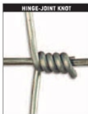
HINGE-JOINT KNOT Can slide horizontally and fold vertically, and is prone to untwisting Typically has less galvanization
